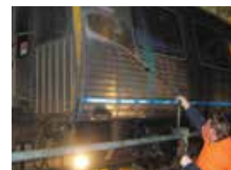
TRANSGEL is used for removing old, thicker, baked on graffiti from trains.
